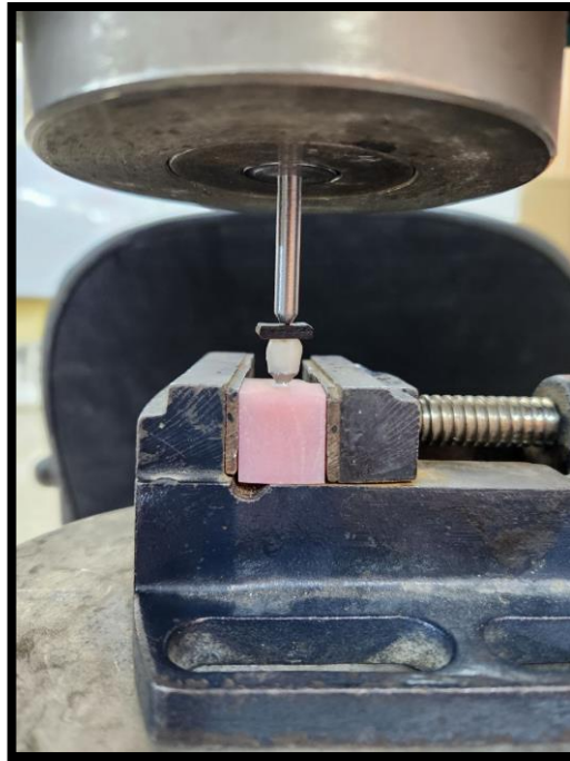
Figure (1-2): crown-abutment combination in LARYEE Universal testing machine)
