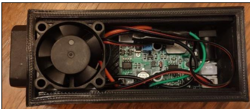
Figure 5: White laser with cooling fan
