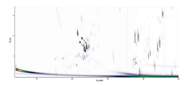
**Figure-1**GC×GC-TOF MScolor plot of the sandalwood powder dissolved in dichloromethane, with the two major constituents highlighted (A)  $\alpha$ -Santalol and (B)  $\beta$ -Santalol.
