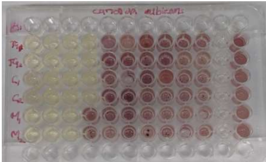
Fig 2: MIC for Ceremagnum plus and Ca(OH) 2 =6.25mg/ml and for MTA=12.5mg/ml
